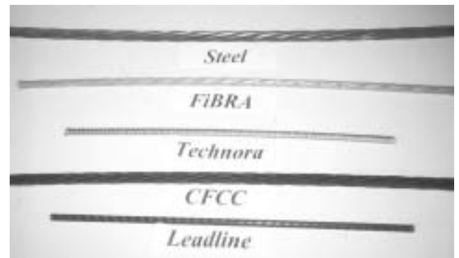
Fig. 1.1—Sample FRP reinforcement configurations.
