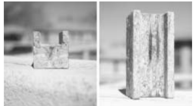
Fig. 4.2—Friction evidence on saddle.
