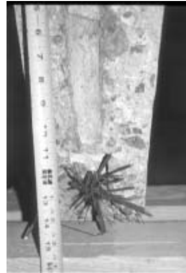
Fig. 4.1—Carbon tendon after “straw broom” failure.
